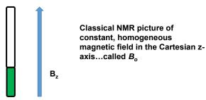
What would happen if, instead of applying a constant field, we applied a GRADIENT field? Transition frequencies will be slightly higher at the top of the tube.
